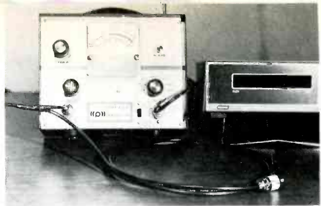
Fig. 4 The worst possible condition is to have a 6-foot coax with nothing connected to the far end. In one case, the output power was reduced to only 0.6 watt.
